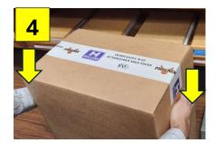
Holland recommends a minimum 3" of tape length down the side of the minor panel of the box. Most water activated tape dispensers have inch length selections - select a length 6" longer than the major panel length and dispense.
