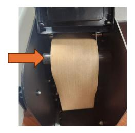
The tape path inside the tape machine is critical for proper dispensing. In most tape machines, there are rollers that guide the tape from the tape roll to the dispensing point. The tape must be threaded over the top of these rollers.
